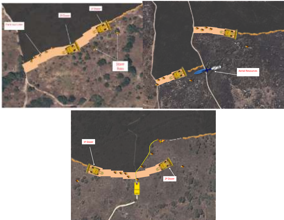
Figure 4. Progress continuous (a), alternative(b) and opposite (c) in direct attack. Source: Juan Caamaño
