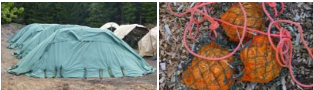
Figure 2: Fleece-covered storage piles (left) and balance bags for the measurement of dry matter losses and changes in moisture content (right)
