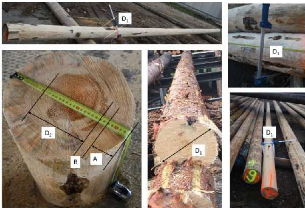
Fig. 5. The analyses example of cross section of infected pine wood pole taken at a conk position, where:
