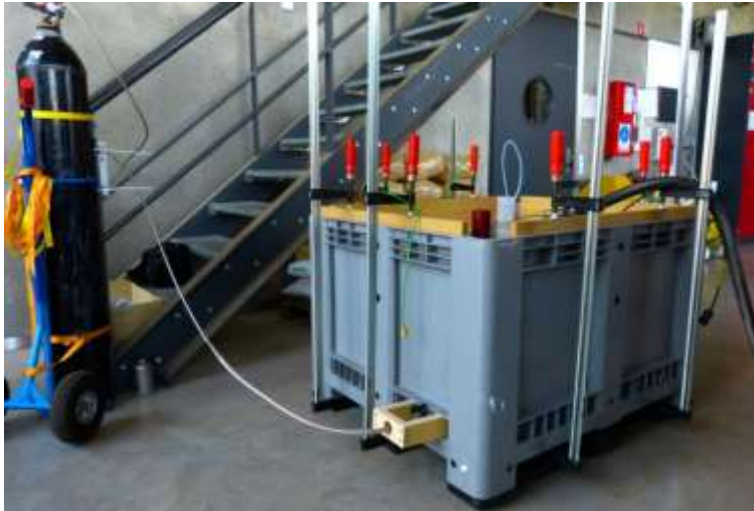
Figure 8: Nitrogen flushing of the anaerobically stored container, with oxygen monitoring at the fermentation bung
