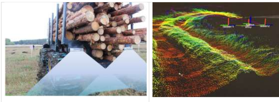
Figure 1 A prototype machine based scanner (left) and resulting point cloud (right)
