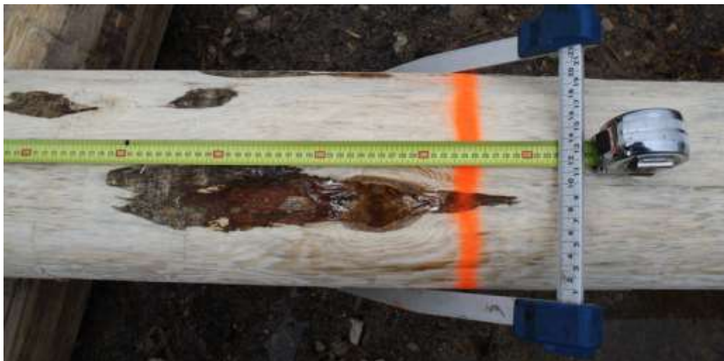
Fig. 3. The measurement of conk location place dimensions on infected wood pole surface
