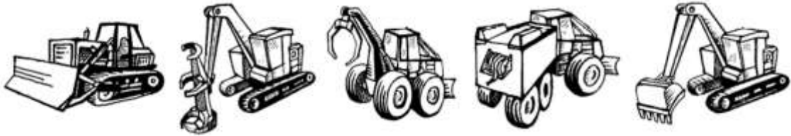
Figure 1: Heavy Equipment Task Force (HETF), common machine types: dozer, feller buncher, grapple skidder, skidgine, excavator. Source: Basko, www.forestoperationsmt.com
