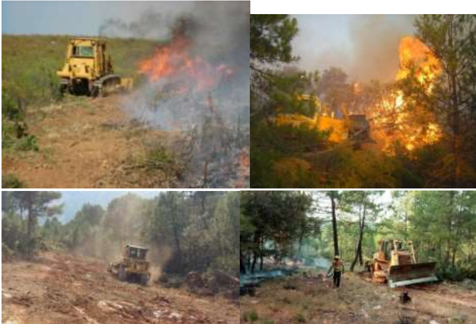
Figures 5, 6, 7, 8: Top left, direct attack in wooded areas. Top right, direct attack shrubs areas. Bottom left, Indirect attack in wooded areas. Bottom right, parallel attack with technical fire maneuvers. Source: Junta de Castilla-La Mancha
