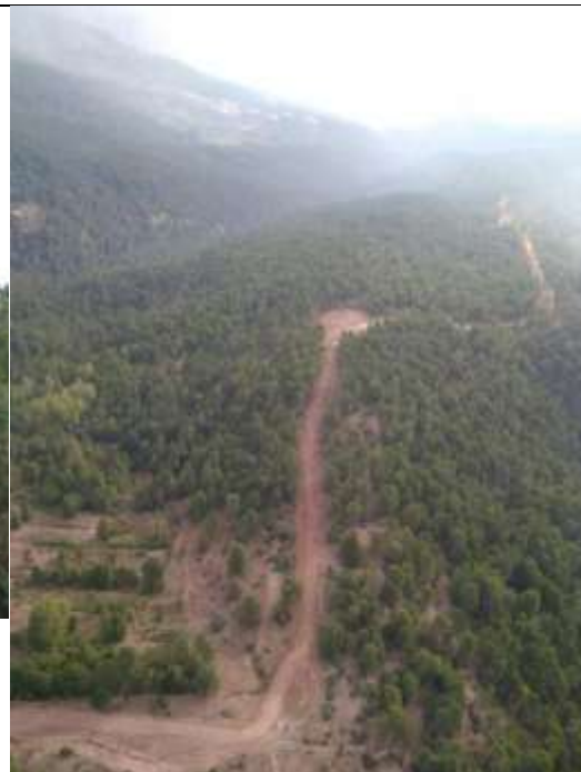
Figure 10: Dozer firelines with logistic platforms and turn around areas and passing bays.
