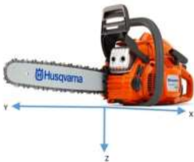
Figure 1. Smart chainsaw and 3D coordinates.
