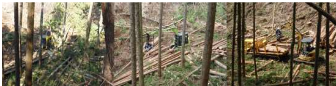
Photo 1 Grapple loader bunching (Left), Processor processing (Middle), and Grapple loader loading to forwarder (Right) at Site A
