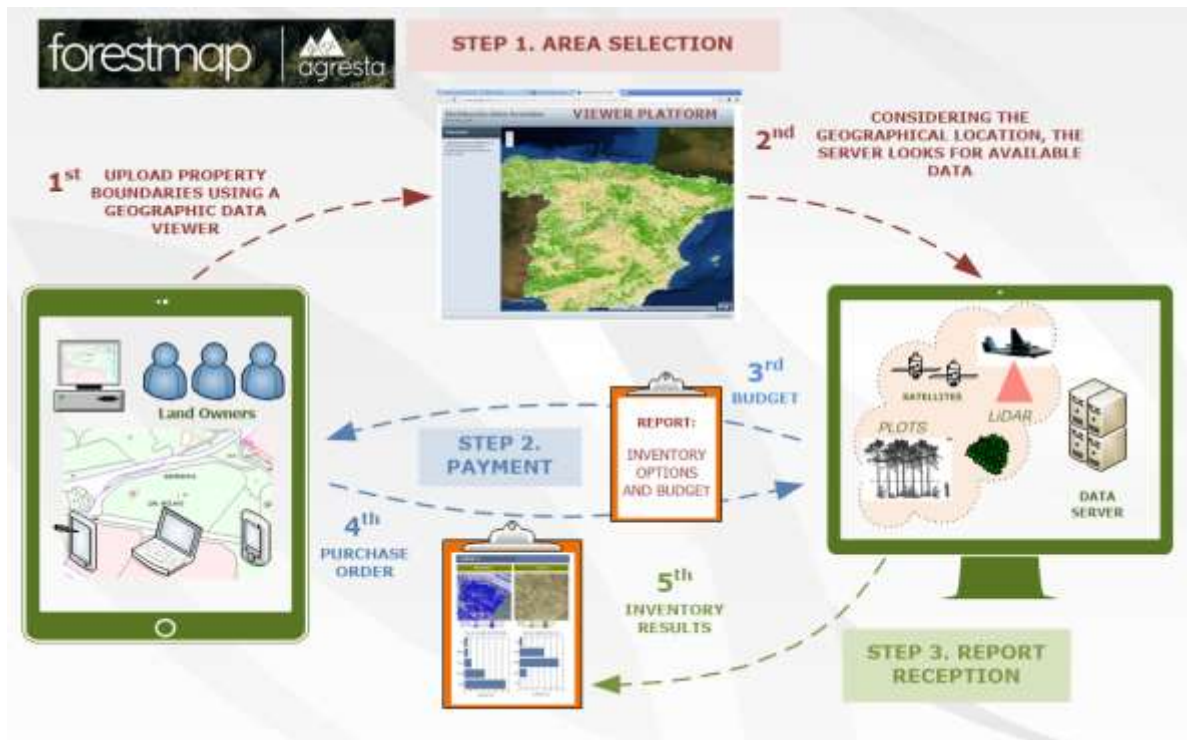
Figure 2 Steps to purchase a forest inventory report for a chosen area. The platform retrieves the necessary information and applies the most convenient models through our implemented algorithm. The platform works in the background to deliver a forest inventory report minutes after payment.
