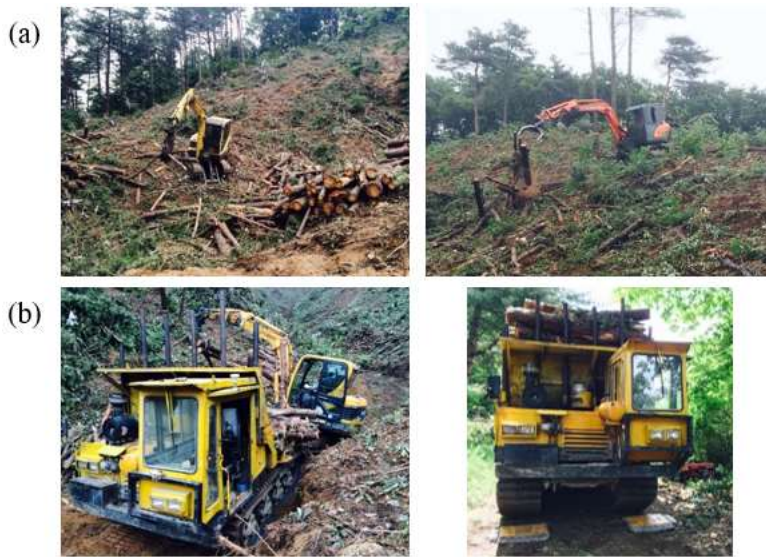
Figure 6. Mechanized extraction with two types of machines: (a) steel-tracked small-shovel and (b) rubber-tracked small-carrier
