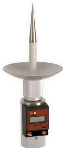
Figure 1. The hand held Wile Bio Moisture Meter (WBMM)(Farmcomp 2018).
